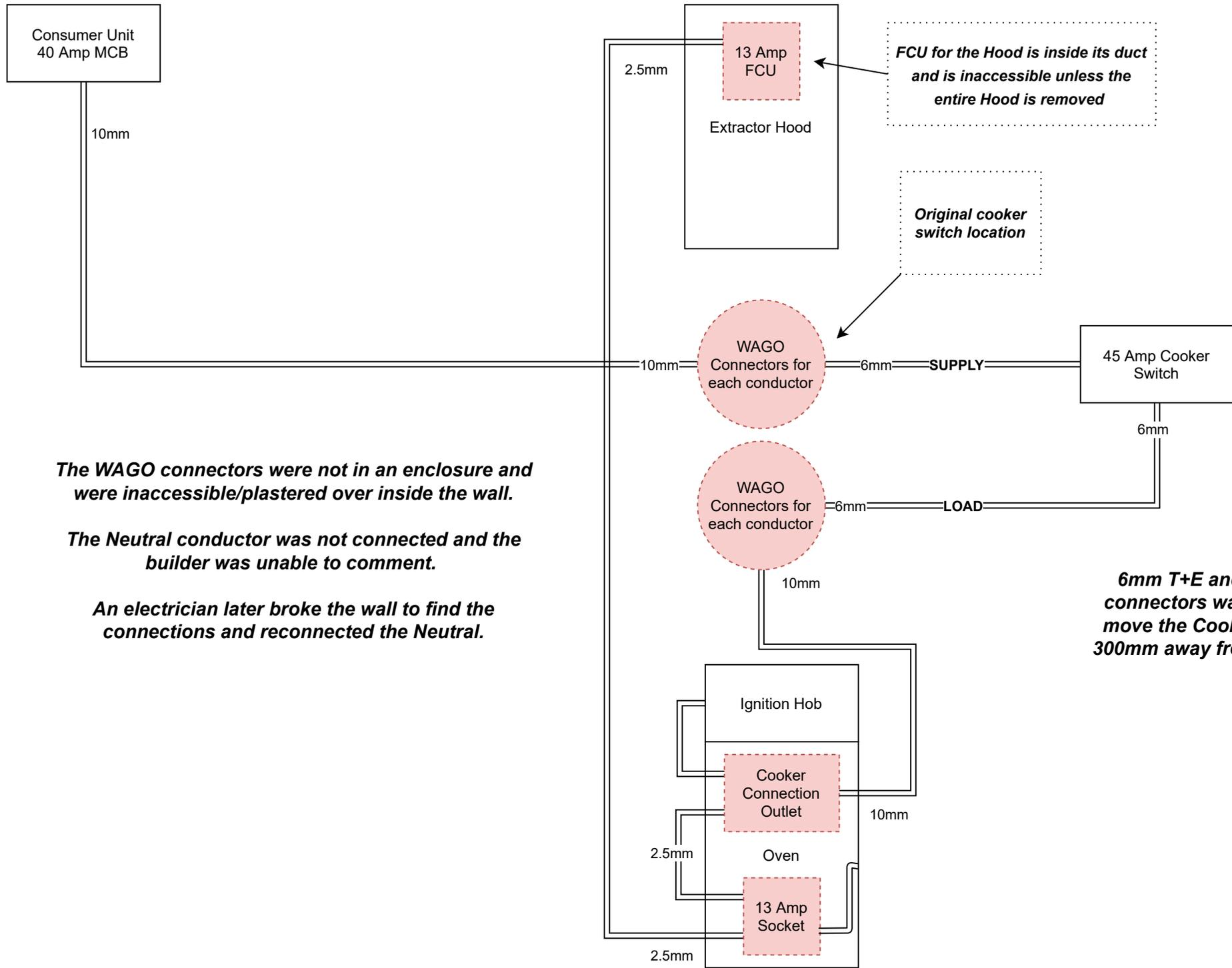
*FCU for the Hood is inside its duct and is inaccessible unless the entire Hood is removed*
